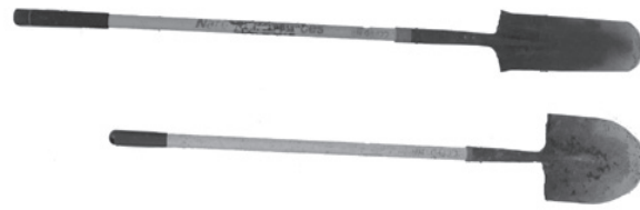
Figure 9.1: Tile spades (top) and round nosed shovels (bottom) are most useful in the field
